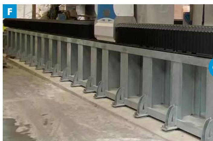
**EN Welded structure plinths**
