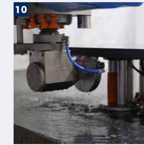
**EN Angle drive for underneath groove**
