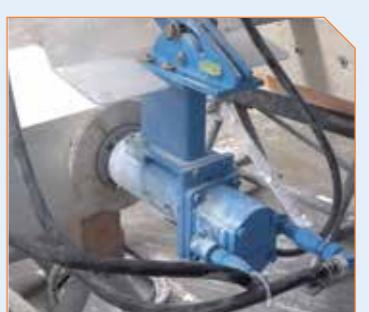
Polishing of a straight edge with angle gear drive.
