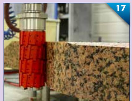
Thick curved edges milling
