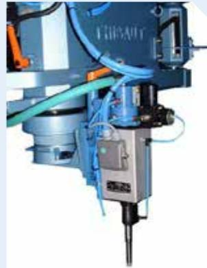
High speed unit 12000 to 18000 rpm
