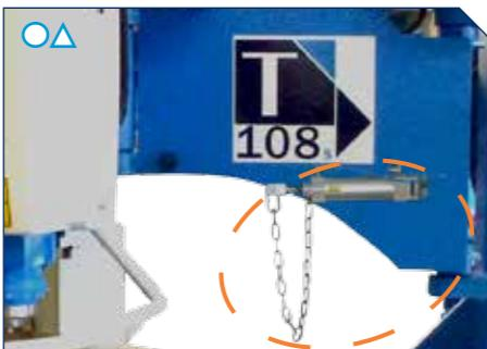
Pneumatic cylinder for side pressure
