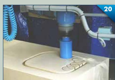
Core drilling in massive limestone
